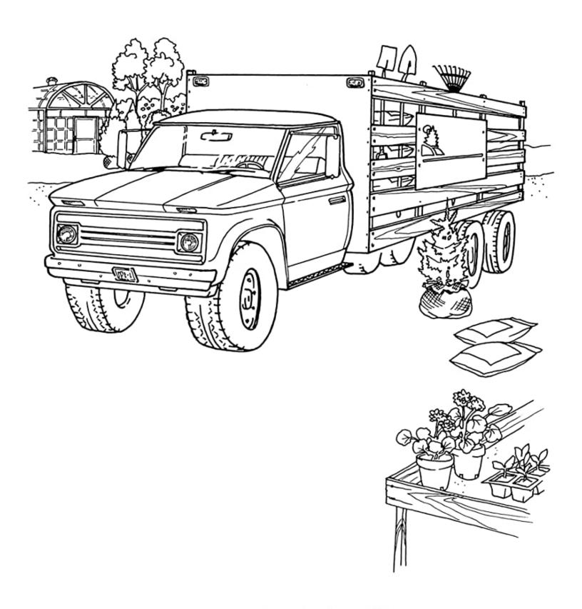
Gardener's Truck. This heavy-duty truck has been adapted for gardening and landscaping duty. It features a platform/stake bed well suited to carry specialized tools and materials to and from distant work sites, as well as two pairs of rear wheels to handle heavy loads.
