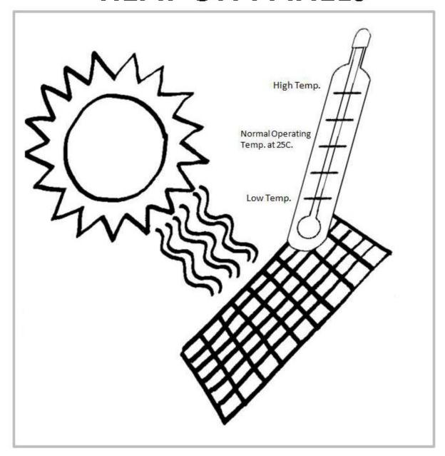
Solar panels power output efficiency can be affected by high atmospheric temperatures. Therefore, investing on panels with low-temperature coefficient is advised.
